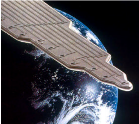
Figure 2: A silicon micromachined probe for recording from individual cells in the central nervous system.
